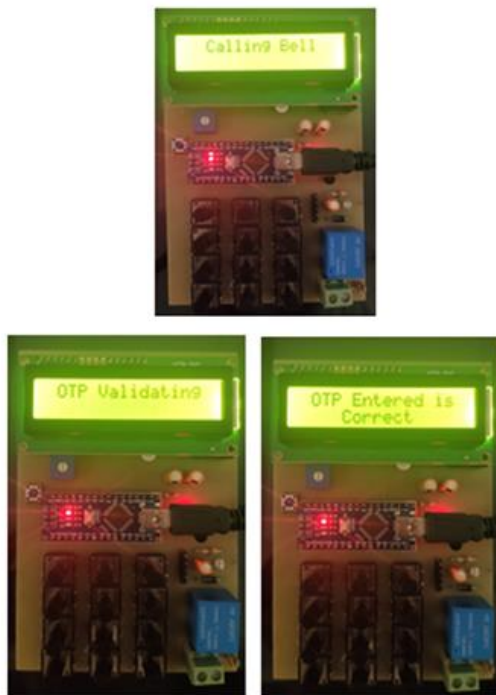
Fig 9: LCD display during ringing the bell, when OTP entered is validated and when OTP entered is correct
