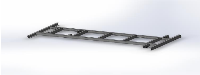
Fig. 2: Design of Chassis created on Solid Works 2017.
