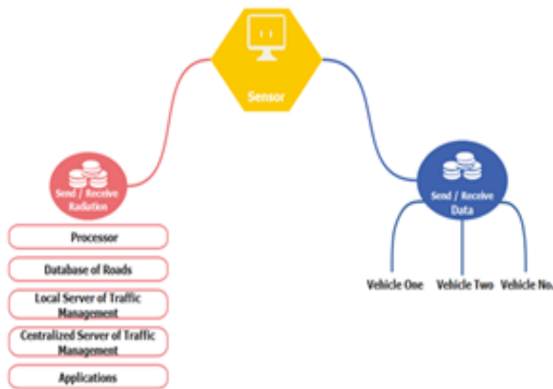
Fig. 11: Communication between LiDAR Sensor and Traffic Management.
