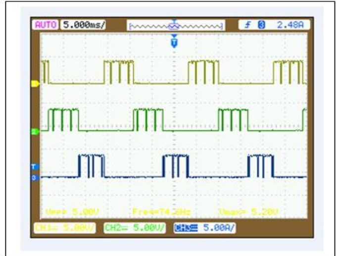
Fig.3.22 Firing pulses for switch 1, 3, and 5 & Firing pulses for switch 4, 6, and 2
