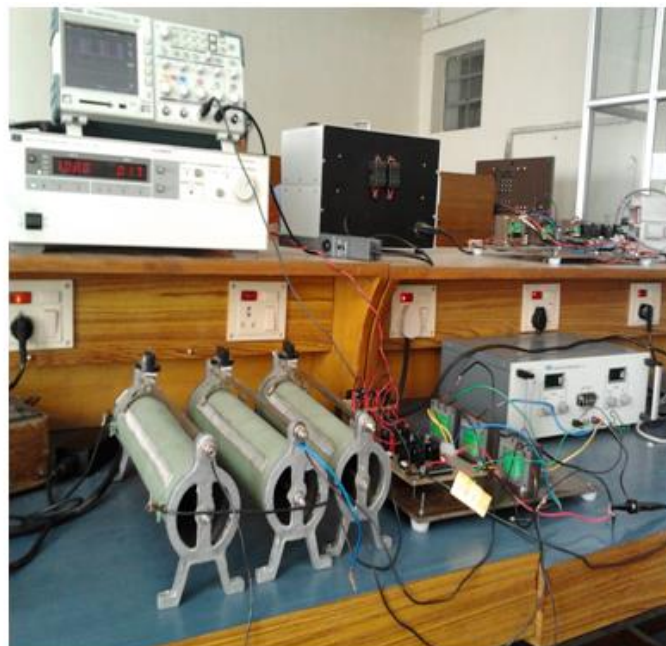
Fig.3.18 VSI with Resistive Load
