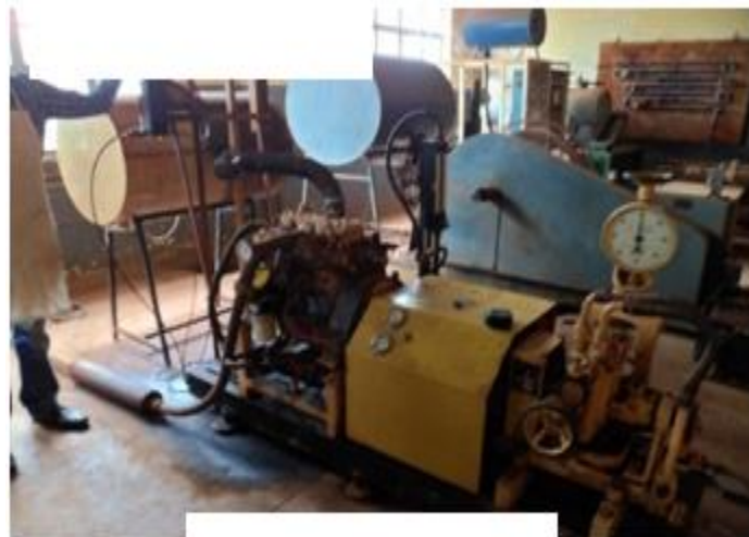
Plate 1: Perkin 4:108 diesel engine mounted on Steady state engine test bed at UNN Nsuka
