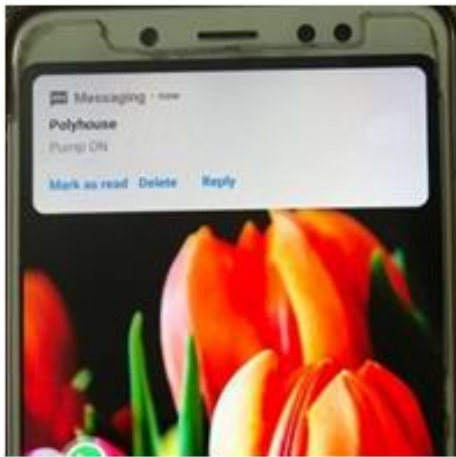
Fig 9:- Figure showing message received during pump ON condition
