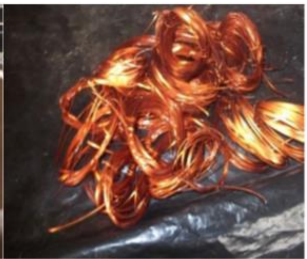
Fig. 14: Flattened copper wire
