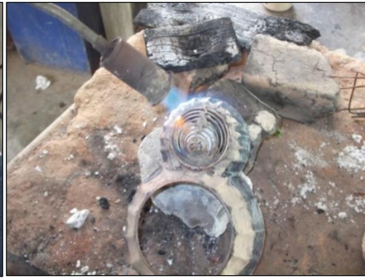
Fig. 53: Soldering of “Gye Nyame”
