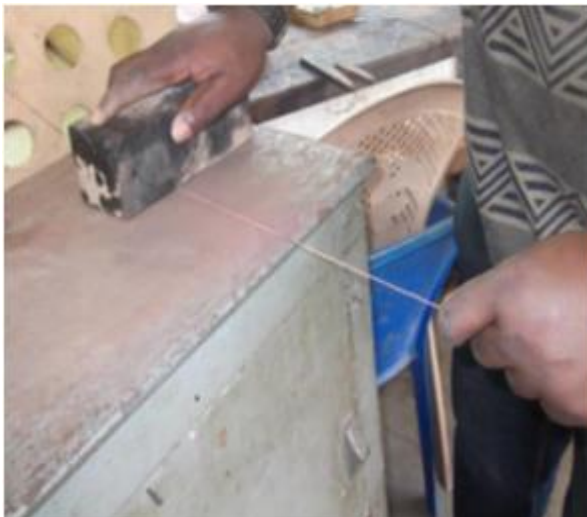
Fig. 15: Twisting of copper wire
