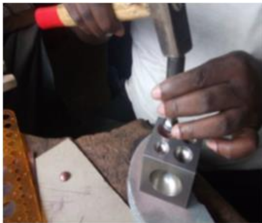
Fig. 19: Doming of spider's body
