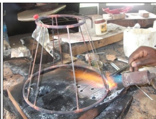
Fig. 56: Soldering of the stakes between the rings
