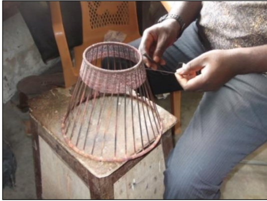
Fig. 57: Plain weave procedure
