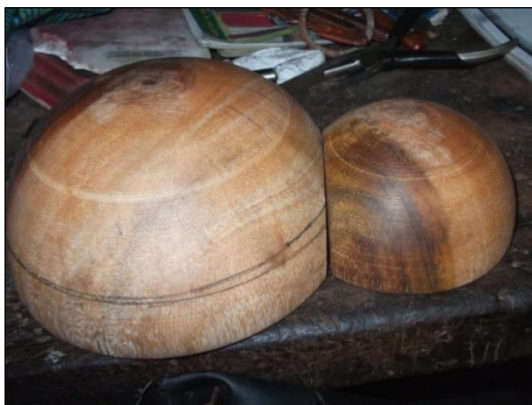
Fig. 48: Wooden mould for the forming of the spider
