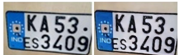
Fig 1:- Low Resolution (LR) Image(left) is enhanced to a high-resolution image(right) using super-resolution (SR). It can be closely observed that the SR image has more texture and clarity as compared to that of the LR image.
