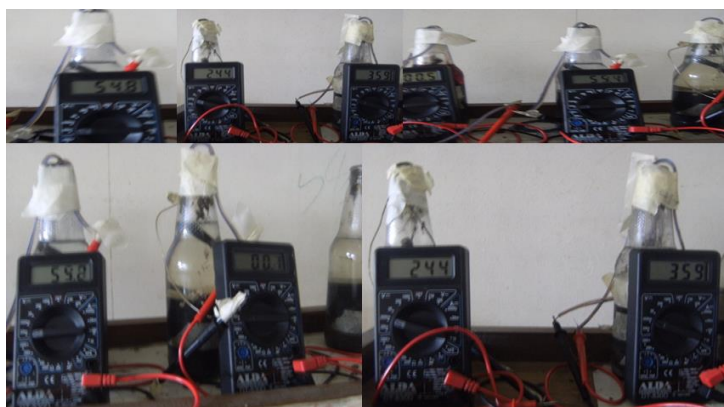
Fig. 2:- Functioning Sediment Microbial Fuel Cells in a Bioelectrochemical system showing voltage of electricity being generated from electron donors in the sediment for investigation.
