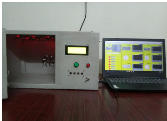
Figure 1: Enose setup fabricated connected with Laptop
