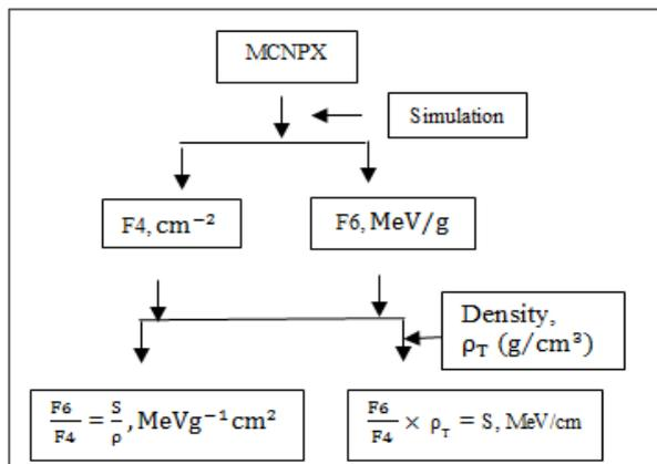
Fig 1:- Schematic Design of the Study Estimates
