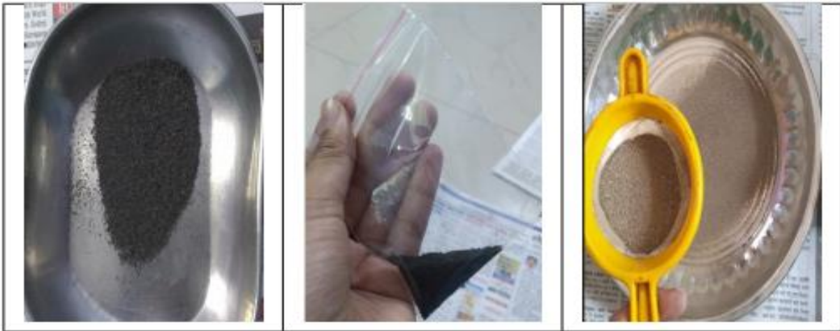
Fig 1:- a) strained brick powder step 1, b) strained brick powder step 2, c) straining of sand.
