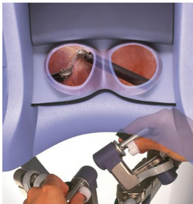
Fig 2 :- da Vinci Vision System. Two tri-CCD cameras provide real 3D vision. The hands are in the.
