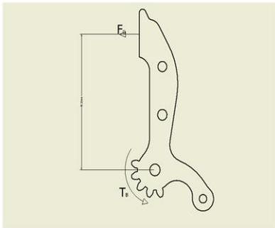
FIGURE 2.18 FORCES ACTING ON GRIPPER
