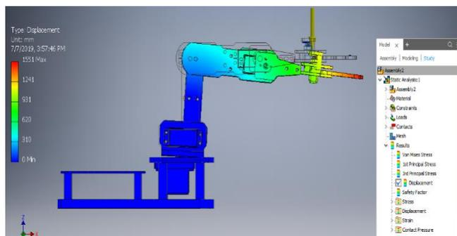
FIGURE 3.2 DEFORMATION AT 50000G LOADING
