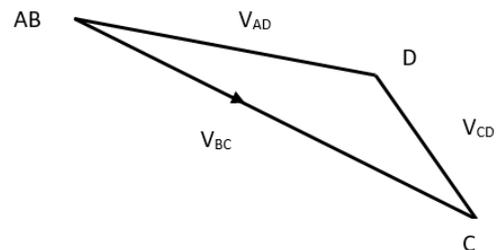
FIGURE 2.17 VELOCITY DIAGRAM OF THE FOUR BAR CHAIN
