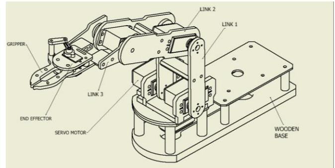
FIGURE 2.22 COMPLETE DIAGRAM OF ROBOTIC ARM
