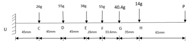
FIGURE 2.12 LOAD DIAGRAM FOR LINK 3
