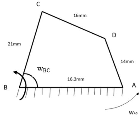
FIGURE 2.16 GRIPPER MECHANISM (FOUR BAR CHAIN)
