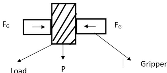
FIGURE 2.19 FRICTION ANALYSIS OF GRIPPER
