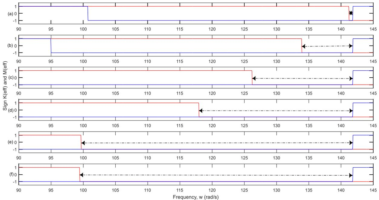
Fig 4:- Plot of signs of effective bulk modulus (blue colour) and mass (red colour) showing increase in double negative frequency bandwidth (denoted by dashed-dotted arrows) due to decrease in value of  $k_1$ ; (a) shows a small DN bandwidth when  $k_1 = k_2 = 25,000 \text{ N/m}$ ; (b) – (f) shows increasing DN bandwidth for constant  $k_2$  (at  $25,000 \text{ N/m}$ ) and  $k_1 = 20,000, 15,000, 10000, 100, \text{ and } 0 \text{ N/m}$  respectively
