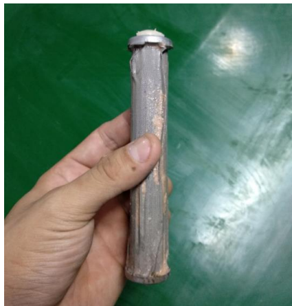
Fig 12 :- An overview of the conditions for the initial improvement of both the Plastisol Dispense Adhesive Process by removing the Pump Machine Filter to facilitate the Plastisol Adhesive flow.
