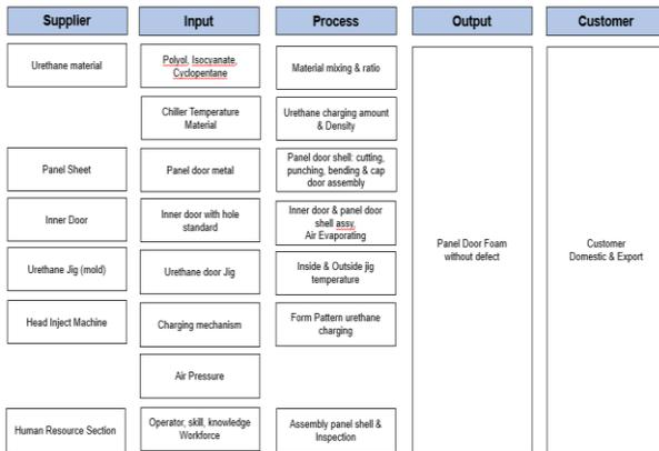
Fig. 1:- SIPOC Diagram for Making Door Process
