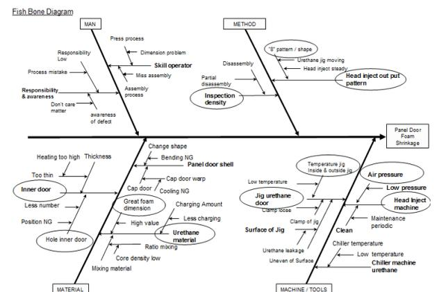
Fig. 3:- Fishbone Diagram Caused of the Damage
